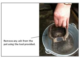
Carefully remove the ash pan and dispose of the ash into a metal container.
