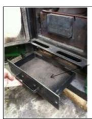
Carefully remove secondary ash pan and dispose of ash into a metal container.
