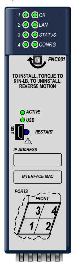
The PACSystems\* RX3i PROFINET Controller module, IC695PNC001 or PNC001, connects a PACSystems RX3i controller to a high-speed PROFINET local area network. It enables the RX3i controller to communicate with I/O devices on the LAN. The PNC001 provides all the functions, services, and protocols required for certification as a PROFINET I/O Version 2.2 I/O Controller, running at both 100 Mbps and 1 Gbps.
