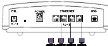
**Figure 5: Any of the 4 Ethernet ports of the AT-AR250E attach directly to a PC Ethernet port or an external Ethernet hub.**
