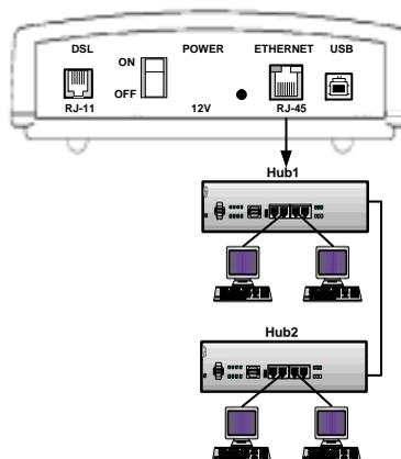
**Figure 6:** Demonstrates cascading hubs using the Ethernet port of the AT-AR240E.
