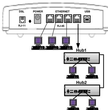
**Figure 7:** Demonstrates cascading hubs using any of the 4 Ethernet ports of the AT-AR250E.
