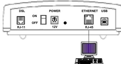
**Figure 4: The AT-AR240E's 10BaseT Ethernet port attaches directly to a PC Ethernet port or an external Ethernet hub.**
