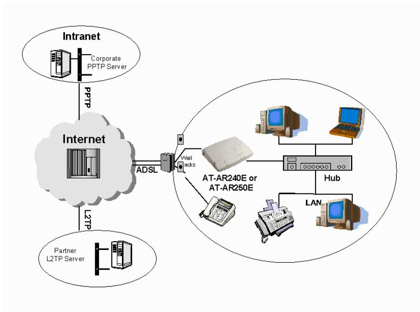
**Figure 11: LAN-to-LAN Connectivity**
