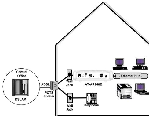
**Figure 8:** For a typical installation, the voice terminals of the splitter are connected to the existing house phone wiring. A separate line is connected from the data terminals of the splitter to a RJ-11 wall jack. The ADSL device is connected through the DSL {RJ-11} jack on the Rear panel to this ADSL {RJ-11} wall jack.
