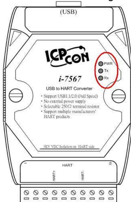
Figure 2-10: LED position of I-7567
