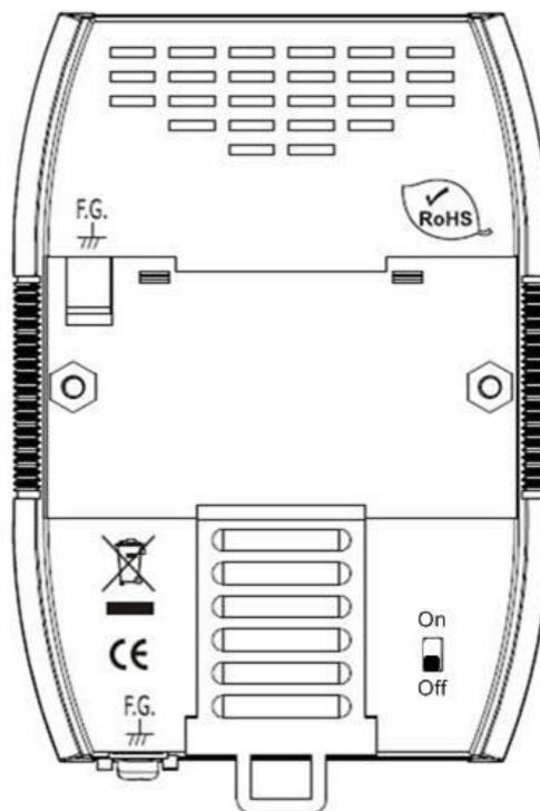
Figure 2-7: Close Internal Resistor
