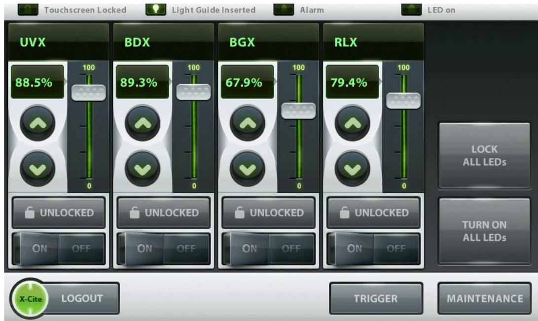
Figure 22 Main LED Screen (Touch Screen Controller)
