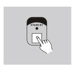
Press Stand By button, its LED blinks, channel 1-4 will be turned off. Press this button again, its LED goes out, channel 1-4 will return to normal mode.
