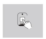
When a chase program is running, you can press Flash buttons 1-4 to select Flash or Latch effect.
