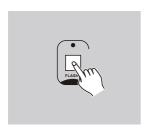
If you want to maintain a channel on, keep pressing the Flash button for 2 seconds, the channel will be turned on regardless of the chase programs.
