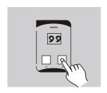
Press Speed UP/DOWN buttons to select chase speed. 01 gives the slowest speed, 99 gives the fastest speed, and the Speed Display shows the current speed.
