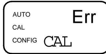
To recalibrate press the MODE key and start the calibration sequence again.
