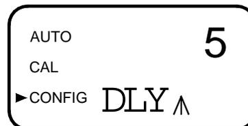
The current selected number of seconds will be shown. Select the desired number of seconds for the "delay on" time for this alarm using the  $\blacktriangle$  and  $\blacktriangledown$  buttons. Once the desired delay time has been set, press the  $\blacktriangledown$  button to accept it.
