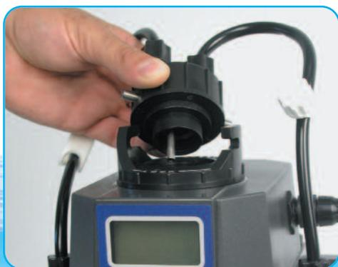
The flow-through sample cell is easily removed to insert a test standard.
