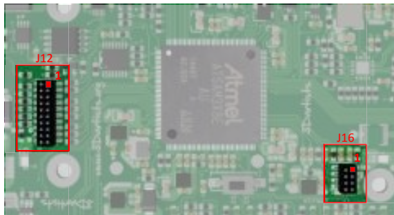
Figure 12 – Piggy Expansion Connectors details
