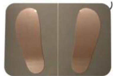
Footwear Electrode for separate shoe testing (350 x 500 x 8mm)
