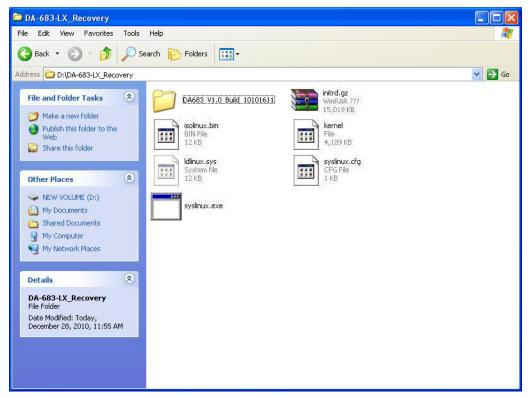
D. Open a DOS prompt and type **D:\syslinux.exe M:** to create a bootable Linux disk. In this example, D: is the USB Disk drive number.
