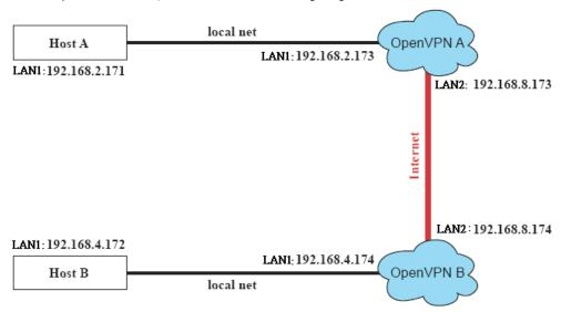
Host A represents the machine that belongs to OpenVPN A, and Host B represents the machine that belongs to OpenVPN B. The two remote subnets are configured for a different range of IP addresses. When this configuration is moved to a public network, the external interfaces of the OpenVPN machines should be configured for static IPs, or connected to another device (such as a firewall or DSL box) first.
