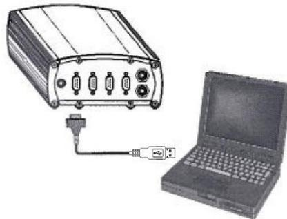
**Figure 6: USB Cable Connection**
