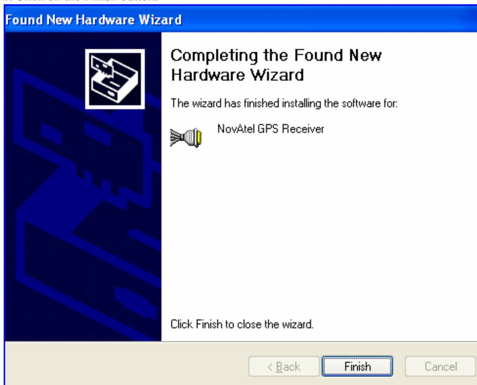
When the system detects the NovAtel USB Virtual Serial Port, the "Found New Hardware Wizard" starts.
