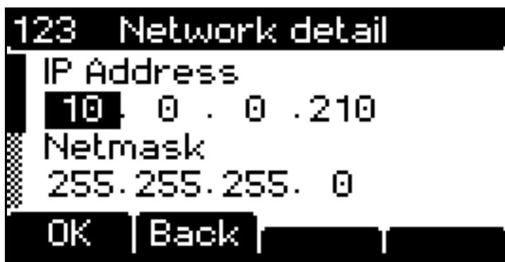
All of the settings for the IP address, netmask, DNS address and gateway must be entered. The numbers are entered using the digits and the up / down keys are used to switch between the entry fields.
