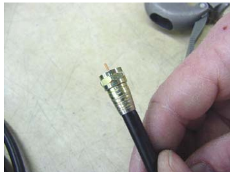
Use a crimping tool to secure the connector to the cable.
