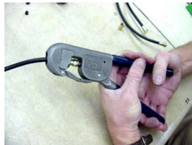
Use a crimping tool to secure the connector to the cable.
