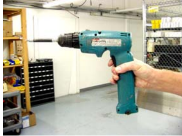
Power Screwdriver - A Short head driver is good for tight situations.
