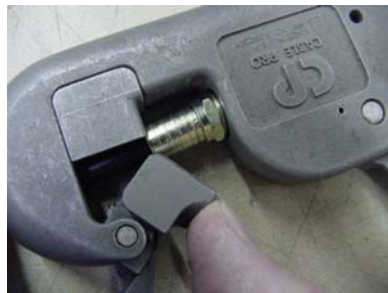
Use a crimping tool to secure the connector to the cable.
