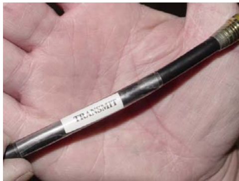
Mark the Transmit cable at both ends.
