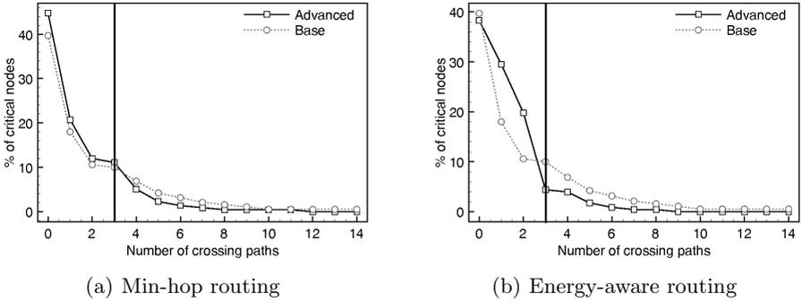
**Fig. 3.** Comparison of the basic and advanced formulations according to the load distribution among critical nodes for both min-hop and energy-aware routing. Area 300m x 300m, 1000 sensor nodes, 70 candidate sites, and  $MAX_{HOPS} = 4$ .
