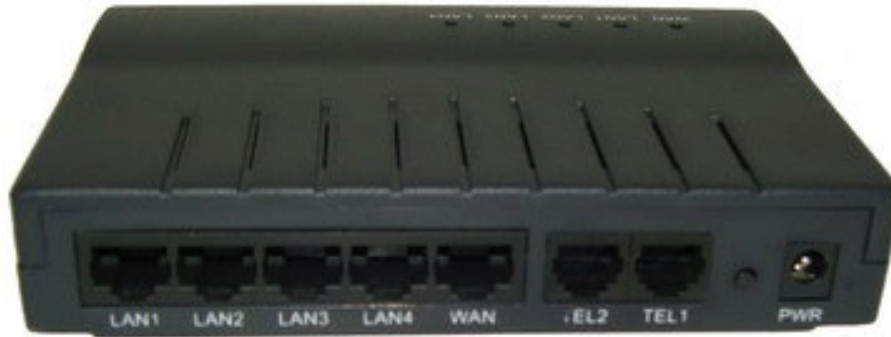
Figure 1-1 ATA hardware overview
