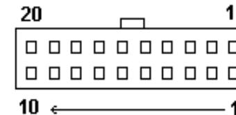
CN3 is a 20-pin ATX Power Supply Connector. Please refer to the following table for the pin assignments.
