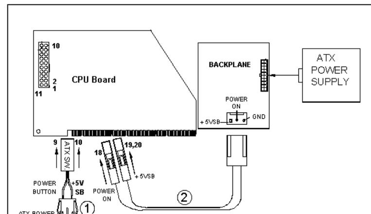
Connect the ATX power supply switch to the pin 9 (power button) and pin 19,20 (+5VSB) of CN2 on the board.
