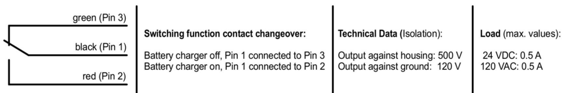
Fig. 7 Connection assignment and technical data for switched output CBL
