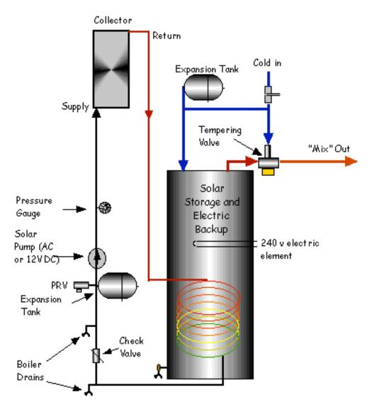
Plumbing diagram of system with one collector, using built-in electric element as backup.
