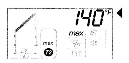
To change high limit, press "Set" for 2 seconds. The current tank temperature will be displayed and "T2" and "Max" flash on the tank. Press "Set" for 2 seconds again until the temperature flashes. Use up or down arrow to change; press "Set" to store.
