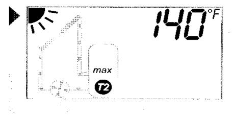
The storage tank has reached the programmed high limit, here set to 140°. "Max" flashes.
