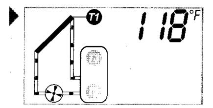
Typical operating screen, with temperature at collectors (T1) displayed. Use arrow to switch to reading storage tank temperature.
