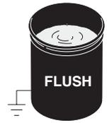
4. Hold a metal part of the gun firmly to the side of a grounded metal pail.
