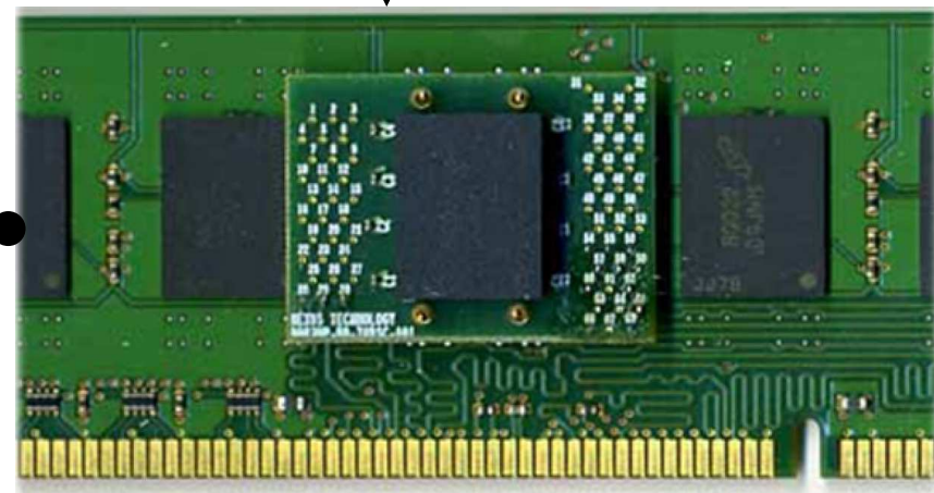
Component Interposer with Chip Interposer on DDR- Module
