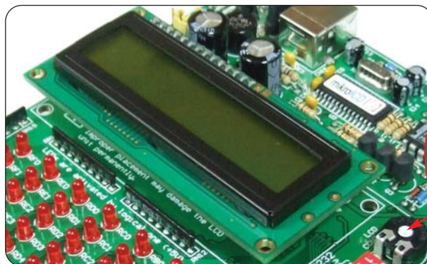
Figure 24. LCD 2x16 in 4-bit mode
