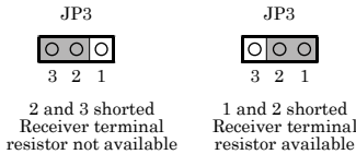
Figure 5.2. Terminal Resistor Settings
