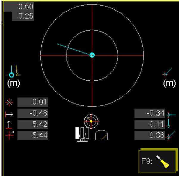
Shows the angle between the feeder and a reference. See details to the right for reference explanation.
