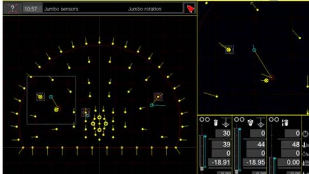
The complete drill pattern is shown. Normal view for the side booms.
