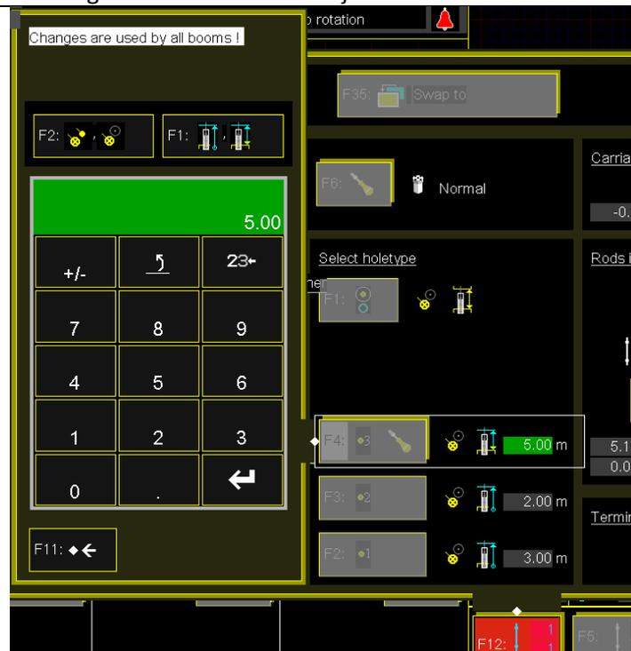
F1: Toggles between measuring from collaring position and reference plane.
