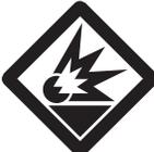
**Never connect to an air source that is capable of exceeding 200 psi.** Over pressurizing the tool may cause bursting, abnormal operation, breakage of the tool or serious injury to persons. Use only clean, dry, regulated compressed air at the rated pressure or within the rated pressure range as marked on the tool. Always verify prior to using the tool that the air source has been adjusted to the rated air pressure or within the rated air-pressure range.
