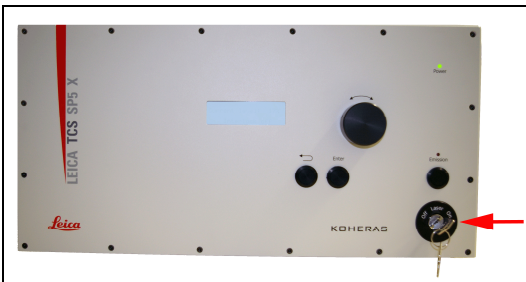
Figure 11: Detachable-key switch for the achromatic light laser
