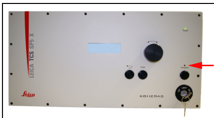
Figure 14: Emission warning indicator at the achromatic light laser
