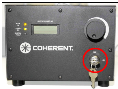
Figure 12: Key switch for the external UV laser
