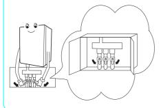
When the boiler is operating, open at least one valve of the distributor.
