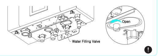
4 When the check lamp on the thermostat turns off and "02" on the temperature indicator window disappears and only the temperature is shown, close the water filling valve by turning it to the right.
