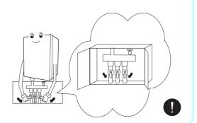
3 Open the water filling valve located on the bottom of the installed boiler by turning it to the left.
