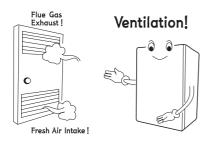
When the boiler takes air from the place where is installed, be sure that the opening ventilation are open.
