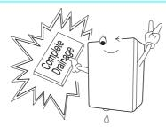
Please completely drain the water from the pipes when not in use for a prolonged period.
