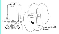
Please leave open distributor valve and gas shut-off valve when not at home for two to three days during the winter.
