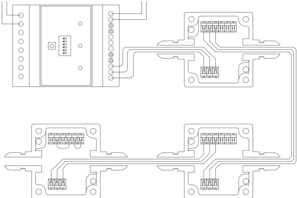
Please note that although a break in the wires connecting the sensors will be detected automatically, in the unlikely event of a sensor failure, there will be no indication of a fault. All Leak Sensors should therefore be tested periodically to confirm that they are functioning correctly by placing the probes in the fluid they are required to detect.
