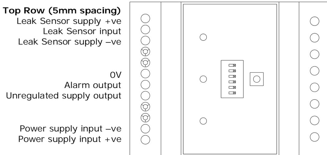
The top row (5mm spacing) has terminals grouped in twos and threes according to function and are used for low-voltage connections only (less than 50V).
