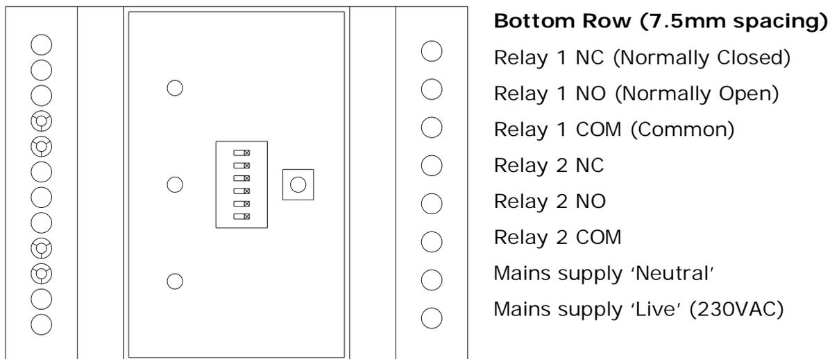
The bottom row (7.5mm spacing) may be used for connecting mains-supply voltages (220V-240V) **or** low voltages if the Controller is not powered by mains. (Mixing mains and low voltages on the bottom row of terminals is not recommended for electrical safety reasons).
