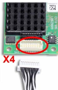
Figure 25: Connecting the Ethernet Assembly Interface (AIFX-RE) to the basic Card NSCP-C100-RE\90E (Example)
