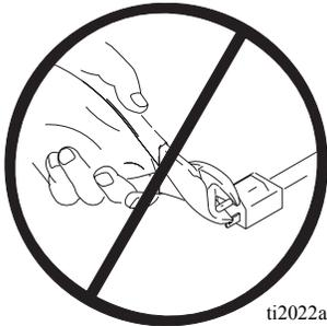
Only use an extension cord with an undamaged 3-prong plug. Recommended extension cords for use with this sprayer are:
