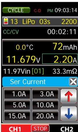
To change the actual charge or discharge current tap the display to the actual discharge current (6). In the lower half of the display appears a selection window.
