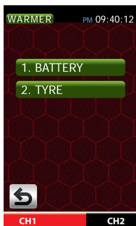
In this sub-menu „HEATING“ you can choose a control program for battery warmer pockets or alternatively a program for the control of tire warmers, by tapping the appropriate icon, in both parts of the program the charger handles both power consumption as well as the control of the connected heater.
