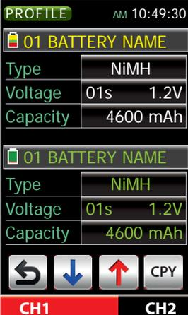
The screenshot shows the 'PROFILE' menu with the time 'AM 10:49:30'. It displays settings for two channels, CH1 and CH2. For each channel, the '01 BATTERY NAME' field is highlighted in yellow. Below the name, the 'Type' is set to 'NiMH', 'Voltage' is '01s 1.2V', and 'Capacity' is '4600 mAh'. At the bottom, there are navigation buttons: a back arrow, a down arrow, an up arrow, and a 'CPY' button. The channel indicators 'CH1' and 'CH2' are shown at the very bottom.
