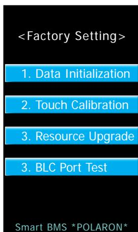
Press and hold the push button placed under the display and turn on the charger. After a short time, the display will appear as shown on the left.
