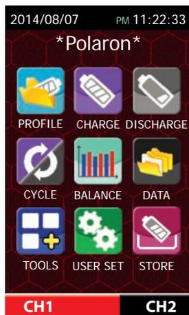
The *Graupner* Polaron charger series are equipped with a touch-sensitive screen. You just have to touch the icon you want to tap or the desired option with a finger or with the pen placed in the right side to go to the desired menu item or to activate the item to set.
