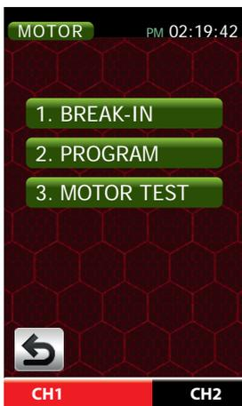
In this sub-menu "MOTOR" you can choose by simply tapping the corresponding icons as break-in program, a motor test program with max. four possible combinations of voltage and duration as well as a motor test program, in all three parts of the program the charger acquires both the power supply as well as the power control of the connected brushed motor.
