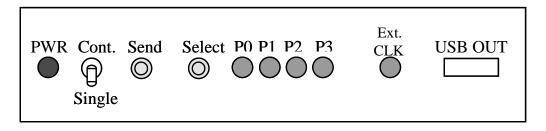
The front panel has one connector, six LEDs, and three switches:
