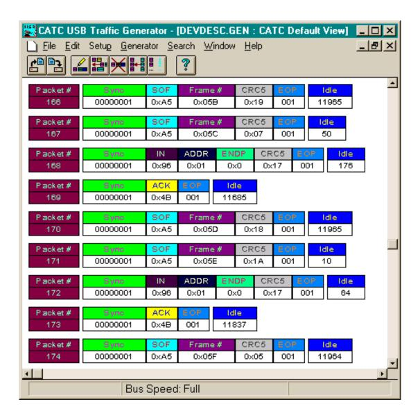
Each field in every USB packet can be separately specified: Sync, PID, Frame #, Addr, Endp, Data, CRC, etc. The length of the idle time between packets can also be defined, and individual bits in any packet changed.
