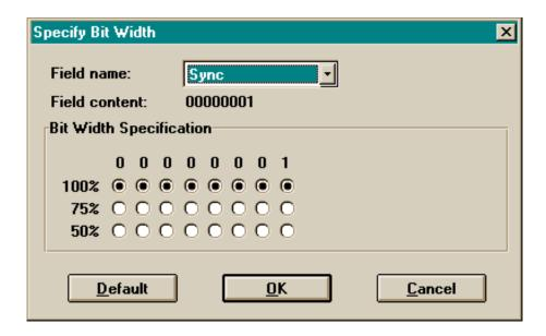
Whether or not such bits are transmitted as so defined, or as normal (100%) width, is further determined when the file is downloaded to the generator box.
