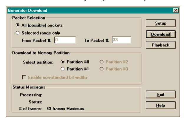
If the current USB traffic file contains bits that have been defined to have non-standard widths (via the Bit Width option in the Add or Modify Packet functions), the "Enable non-standard bit widths" check box will be enabled. A mark in this box will preserve the non-standard widths as they are loaded into the generator box; clearing the box will load only standard (100% width) bits into the generator box (though the computer-resident file will not be modified).
