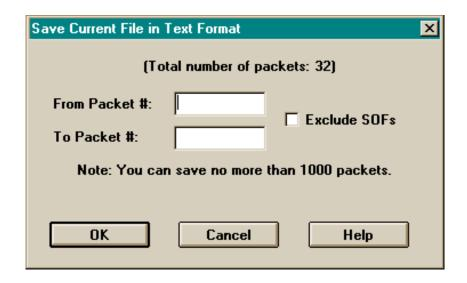
Up to 1,000 packets can be saved at a time. The operator can elect to save SOF packets or exclude them from the text file. The saved file can be opened with any standard text editor.
