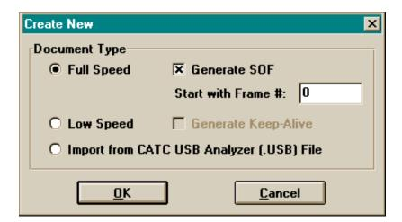
The new file may be opened as an empty file, allowing the operator to specify packets one by one, by **clearing** the "Generate SOF" check box (or, in low-speed mode, by clearing the "Generate Keep-Alive" check box). Another option is opening the file with pre-existing start of frame packets, by **marking** the "Generate SOF" check box (or, in low-speed mode, with pre-existing EOP packets, by marking the "Generate Keep-Alive" check box). In this way, custom
