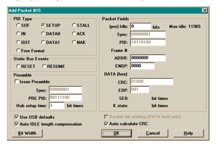
Only relevant fields can be modified. Start with the PID Type field: the appropriate fields for the selected PID type will subsequently become active. For example, for the SETUP packet shown above, the FRAME # and the DATA field are not activated. If the PID is changed to SOF, the FRAME # field becomes active. For DATA0 and DATA1 PIDs, the DATA field becomes active.
