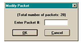
When the packet number selection is confirmed, a dialog box (almost identical to that used by Add Packet, though initialized to display the current data) opens, enabling modification of the various fields of the chosen packet.
