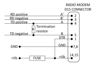
$FUSE = 1 \text{ A slow } (+6 \dots +30 \text{ V assembly}) \text{ or } 2.5 \text{ A slow } (+3 \dots +9 \text{ V assembly})$
