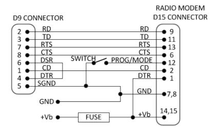
FUSE = 1 A slow (+6 ... +30 V assembly) or 2.5 A slow (+3 ... +9 V assembly) SWITCH = Programming mode switch (ON=Programming mode, OFF=Data transfer mode)
