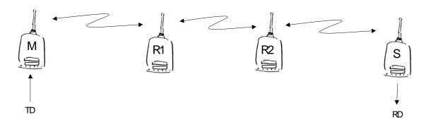
When using repeaters, the same packet is sent via a (radio) channel several times. A radio modem situated in the repeater chain will often hear other radio modems in addition to the immediate neighbouring radio modems. With Source Mode Routing the complete address
