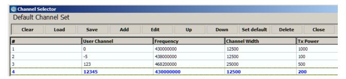
SL commands provide an interface for a host device to command the radio modem directly. An example of the procedure for creating or replacing a channel list:
