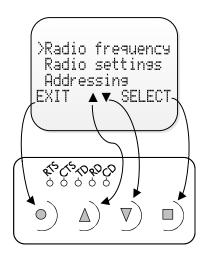
Pressing DOWN ( $\nabla$ ) button the cursor moves downwards. Depending on the sub-menu, the button also scrolls the digits of numerical values when changing some settings.
