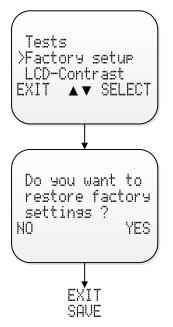
Enter the settings menu first by pressing SETUP button (■) on the top level view.
