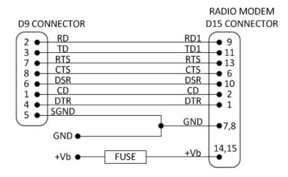
$FUSE = 1 \text{ A slow } (+6 \dots +30 \text{ V assembly}) \text{ or } 2.5 \text{ A slow } (+3 \dots +9 \text{ V assembly})$
