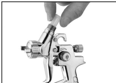
Figure 3. Installing filter into Model H8117.
