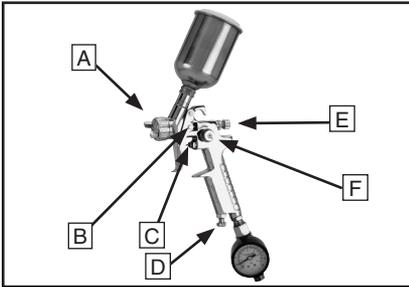
**Figure 15.** Lubrication points.
