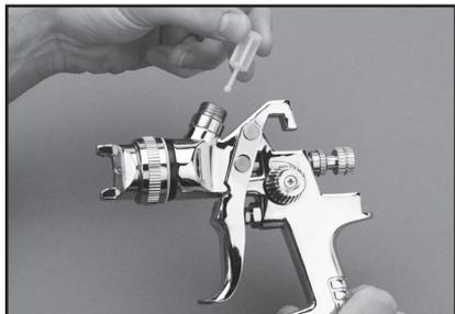
**Figure 3.** Installing filter.
