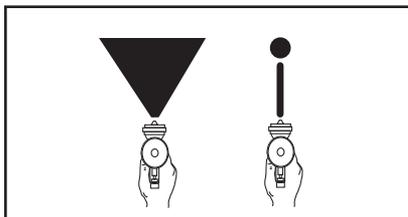
**Figure 9.** Fan adjustment.
