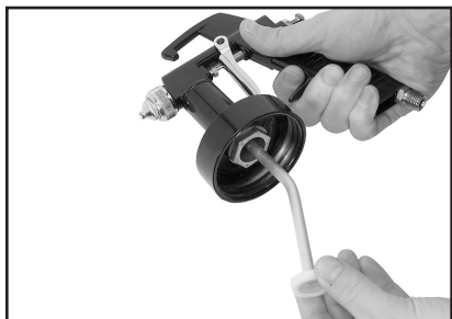
Figure 4. Installing H3254 filter.
