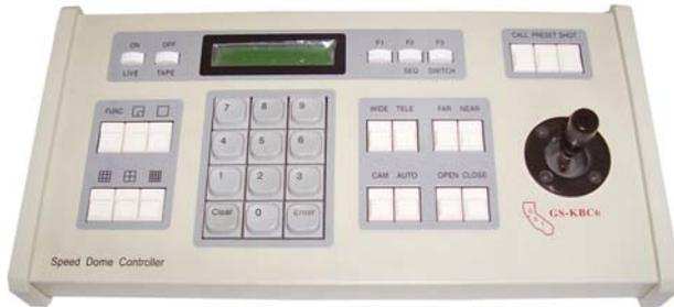
This intelligent spherical video camera can be connected to keyboard or special control equipment via RS485. The process of up and down and left and right movement of the video camera, and the lens zooming can be remote controlled.
