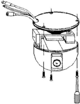
(4) Install the spherical housing on the base plate of the video camera according to the figure and then, push the decoration ring up into the slot.
