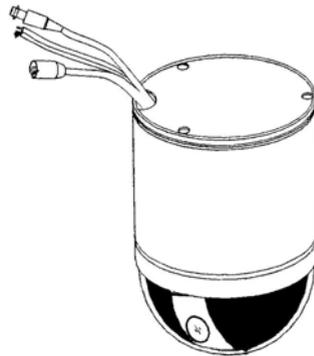
(3) Fix the base plate of the video camera on the ceiling plate with 3 screws.
