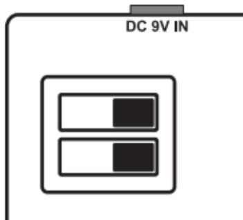
**True Bypass** – is a hard-wire bypass that gives absolutely no coloration of tone when the pedal is bypassed. Using True Bypass on all pedals is a perfect choice in setups with a few pedals and relatively short cables before and after the pedals.
