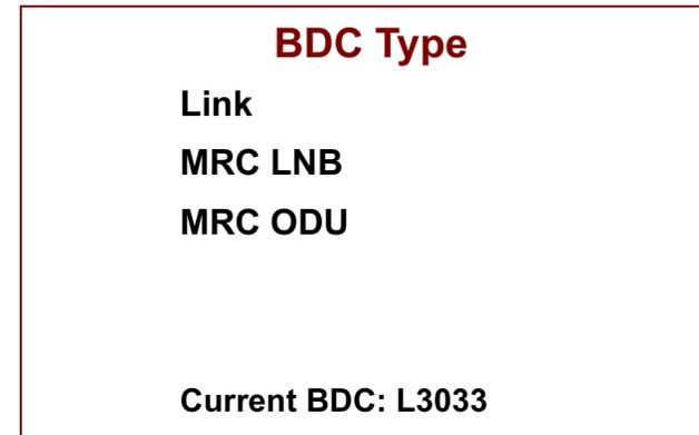
2. Determine the model number of the downconverters that are connected to the receiver and select the appropriate menu option. This displays a list.
