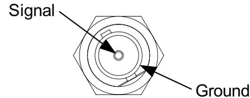
**CV 1, CV 2** The Composite Video (CV) connectors are 75 ohm, female, BNC connectors that output an analog video signal.
