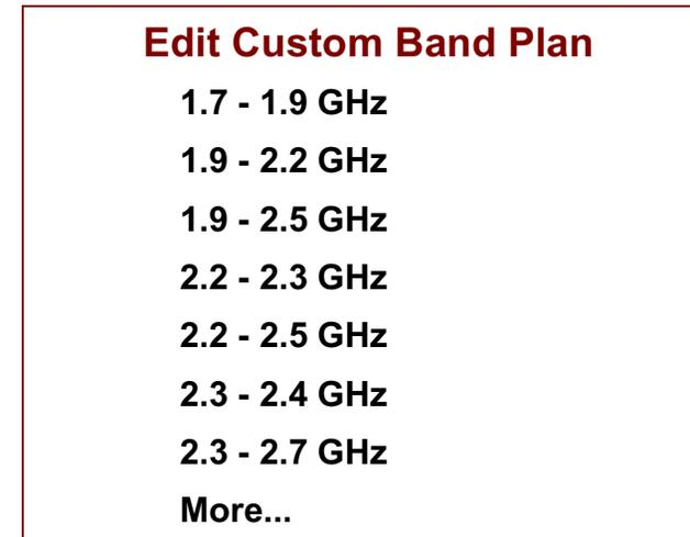
4. Select the band plan that you need to modify or select **More** to display more RF bands. This opens the **Edit N GHz Custom Plan** menu similar to [Figure 3-32 on page 3-28](#), where “N” is the RF band you selected. This screen consists of channel numbers down the left side and three columns of frequencies (for the minus offset, center frequency, and plus offset). Since these are to be custom frequencies, the task is to change all the values to match your operating conditions.
