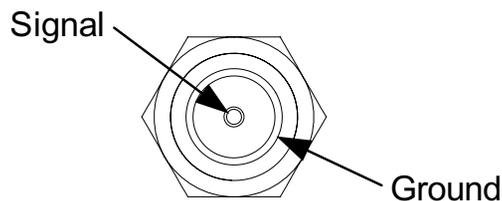
**BDC 1 to BDC 6** The Block Downconverter (BDC) connectors are 50 ohm, TNC connectors that accept the UHF signals from the downconverters and their corresponding antennas.
