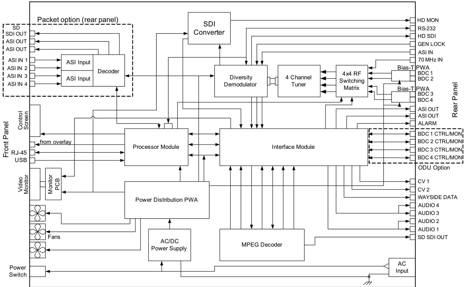
Each BDC operates by mixing a Local Oscillator (LO) signal together with the incoming RF signal and producing a UHF output signal in the range of 110 to 860 MHz. The incoming signal is filtered and then amplified by a Low Noise Amplifier (LNA) and is sent along to the mixer. See [Figure 7-2](#) for a functional block diagram of the block downconverter circuitry.
