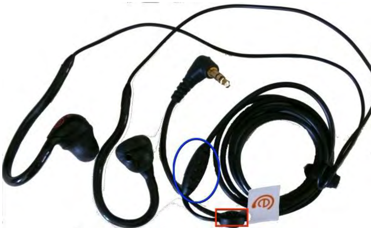
Figure 1. The PCS-100 earphones have a 50" cable with highly flexible ear loops at one end and a standard 3.5mm gold-plated stereo jack at the other. A plastic splitter (blue oval) without a microphone or remote controls (volume; pause/play) is located about 11.5" below the bottom of the ear loops. A plastic slider (red rectangle) above the splitter helps minimize audio artifacts due to movement.
