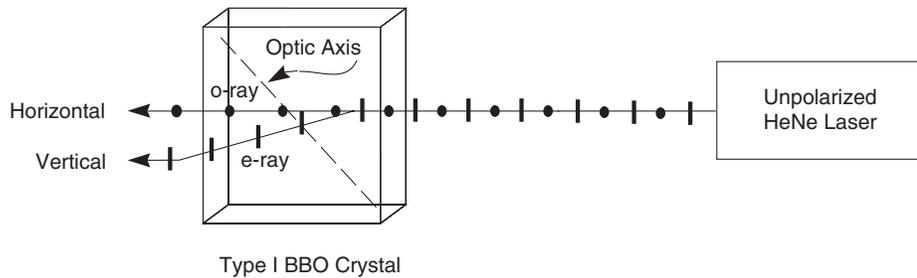
**Figure 5-5: Unpolarized light from a HeNe laser shown entering a birefringent crystal, such as BBO.**
