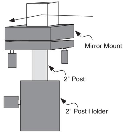
**Figure 5-1: A Typical Right-angle Turning Prism Assembly**
