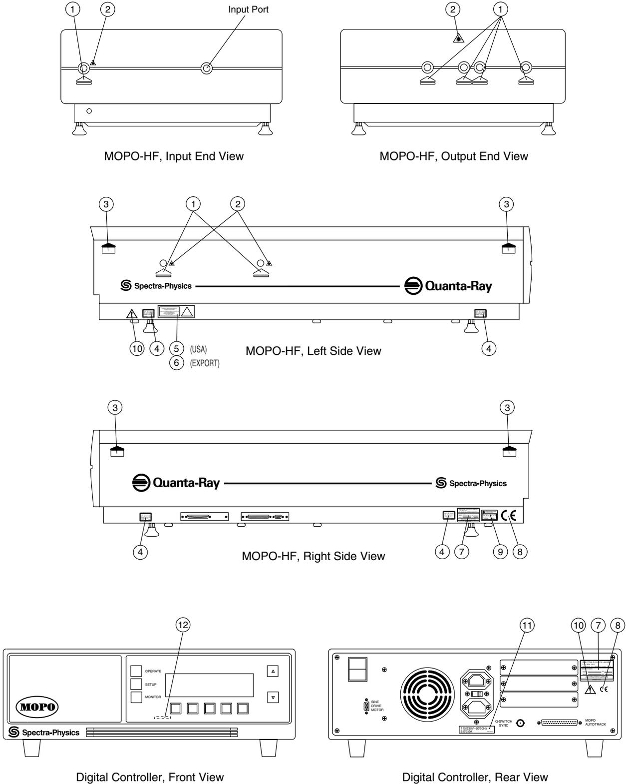
Figure 2-3: CE/CDRH Radiation Control Drawing
