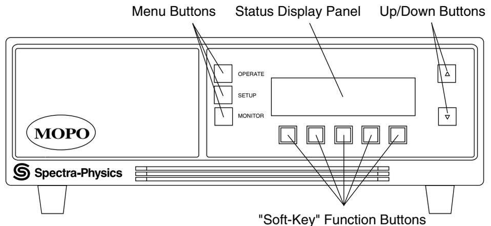
Figure 4-3: The Digital Controller Front Panel
