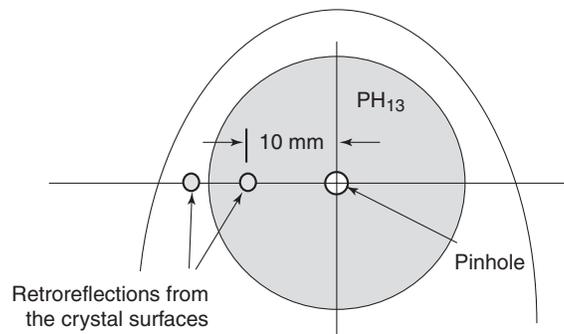
**Figure A-5: The HeNe beam retroreflections from the crystal as seen on PH<sub>13</sub> for cases A and C.**
