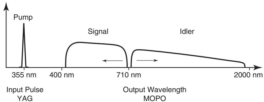
**Figure 3-3: Theoretical signal and idler Output wavelengths for 355 nm Pump**
