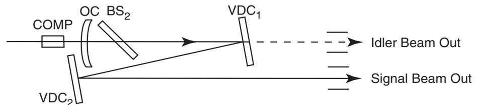
**Figure 3-8: Dichroic Beam Separation**
