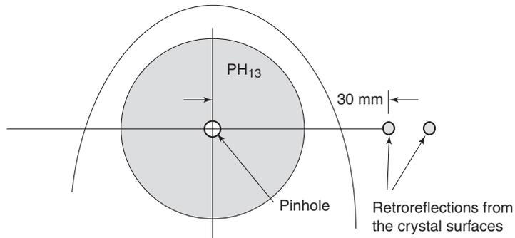
**Figure A-6: The HeNe beam retroreflections from the crystal for case B.**
