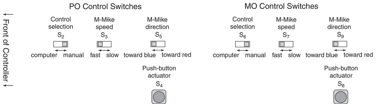
**Figure D-1: The Autotrack control pc board motor mike switches.**
