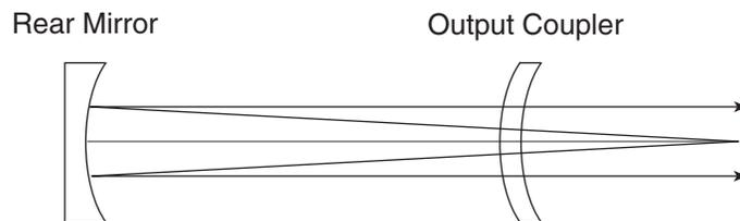
**Figure 3-6: Schematic of an Unstable Resonator Design used in the *MOPO-HF* Series.**
