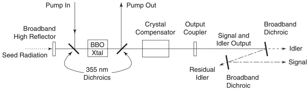
**Figure 3-7: Power oscillator cavity geometry. Illustration shows separation of signal and idler output beams with broadband dichroic mirrors.**
