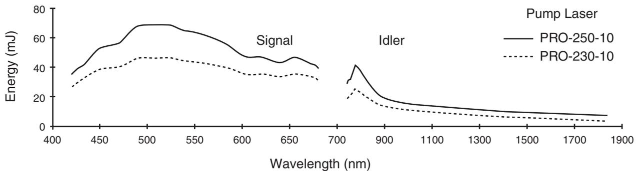
Figure 3-10: *MOPO-HF* Turning Curves
