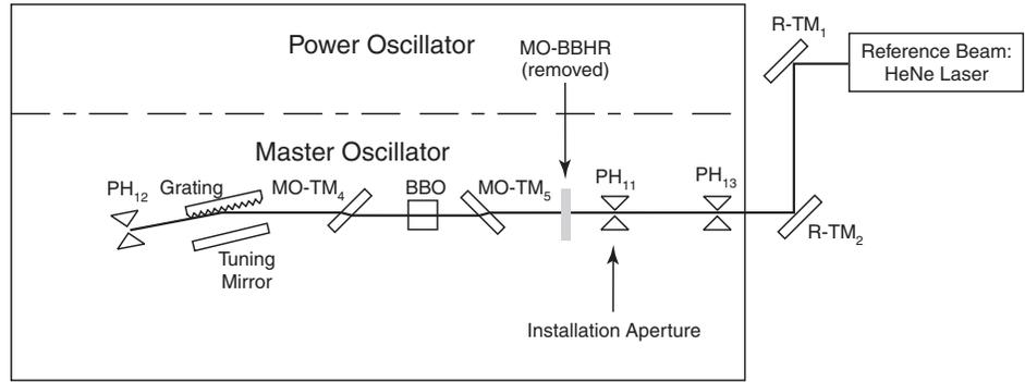
**Figure 5-4: Reference beam alignment for the master oscillator. MO-BBHR is removed to allow the reference beam into the optical cavity. For purposes of clarity, some optical components have not been shown.**
