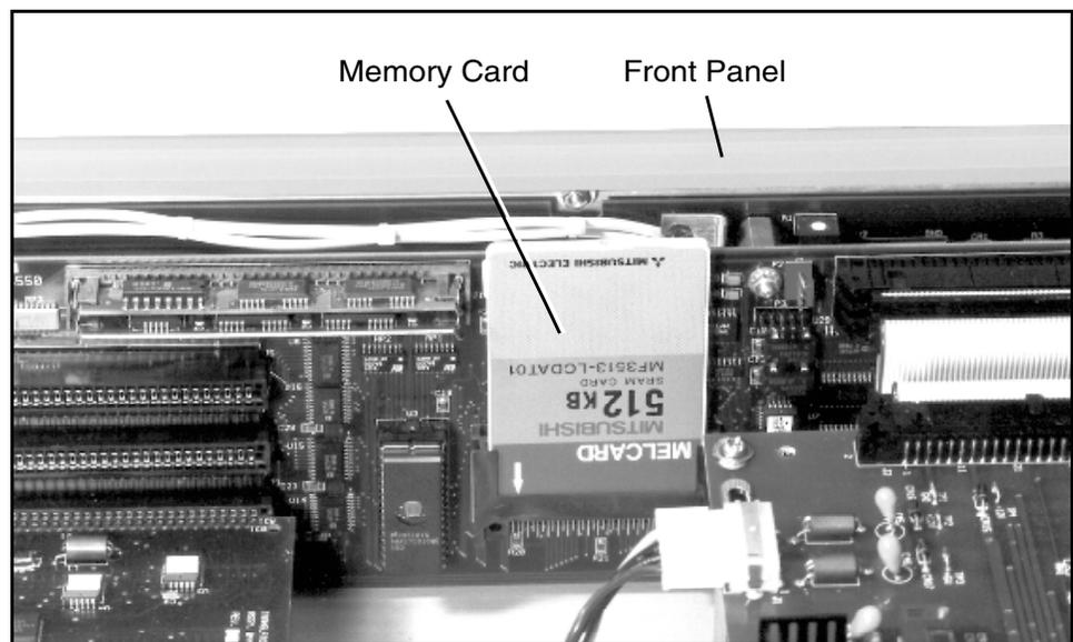
**Figure F-1:** Electronics unit showing location of removable PCMCIA memory card.
