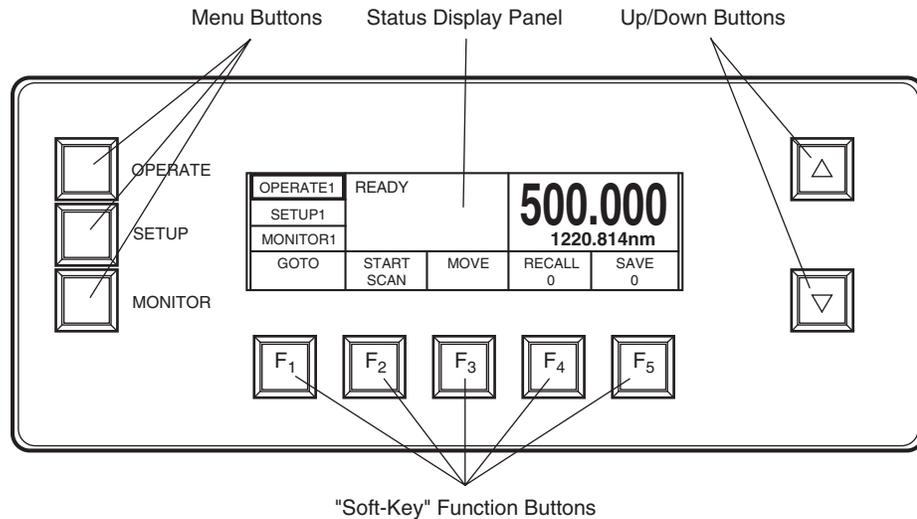
Figure 6-1: Initial configuration of the electronics panel
