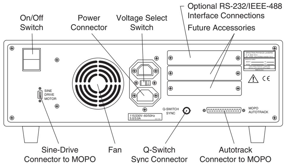
**Figure 4-4: The Digital Controller Back Panel**
