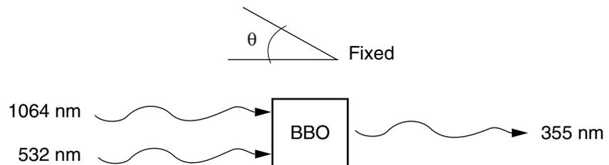
**Figure 3-1: Frequency mixing to generate the third harmonic of Nd:YAG**
