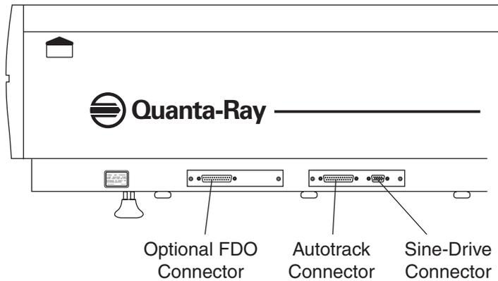
Figure 4-2: MOPO-HF Connectors, Right Side View
