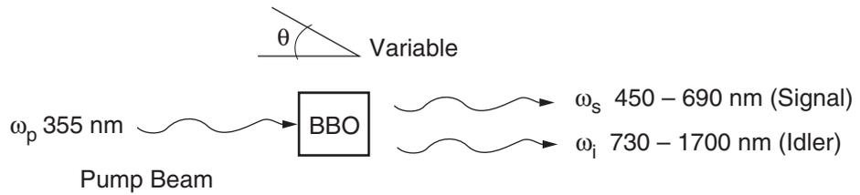
**Figure 3-2: Parametric Amplification to Generate Tunable Output from 450 nm to Beyond 1700 nm.**
