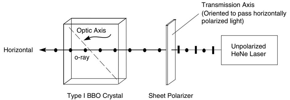
**Figure 5-6: Horizontally polarized light passing through a birefringent crystal, such as BBO.**
