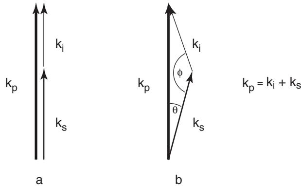
**Figure 3-9: Collinear (a) and noncollinear (b) phase matching**
