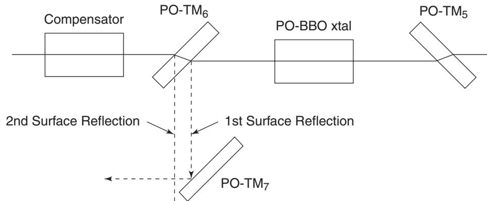
**Figure 5-22: Alignment of the first surface reflection from PO-TM<sub>6</sub> onto PO-TM<sub>7</sub>.**
