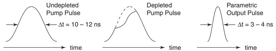
**Figure 3-5: Pump pulse depletion and resulting parametric output pulse.**
