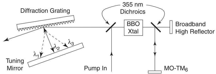
**Figure 3-4: The MOPO-HF Master Oscillator uses a Grazing Incidence geometry to produce sub 0.075 cm<sup>-1</sup> mean linewidths. The wavelength centered at the peak of the BBO gain bandwidth,  $\lambda_2$ , is reflected back into the cavity, while those at the edge of the gain bandwidth walk out of the cavity and do not oscillate.**
