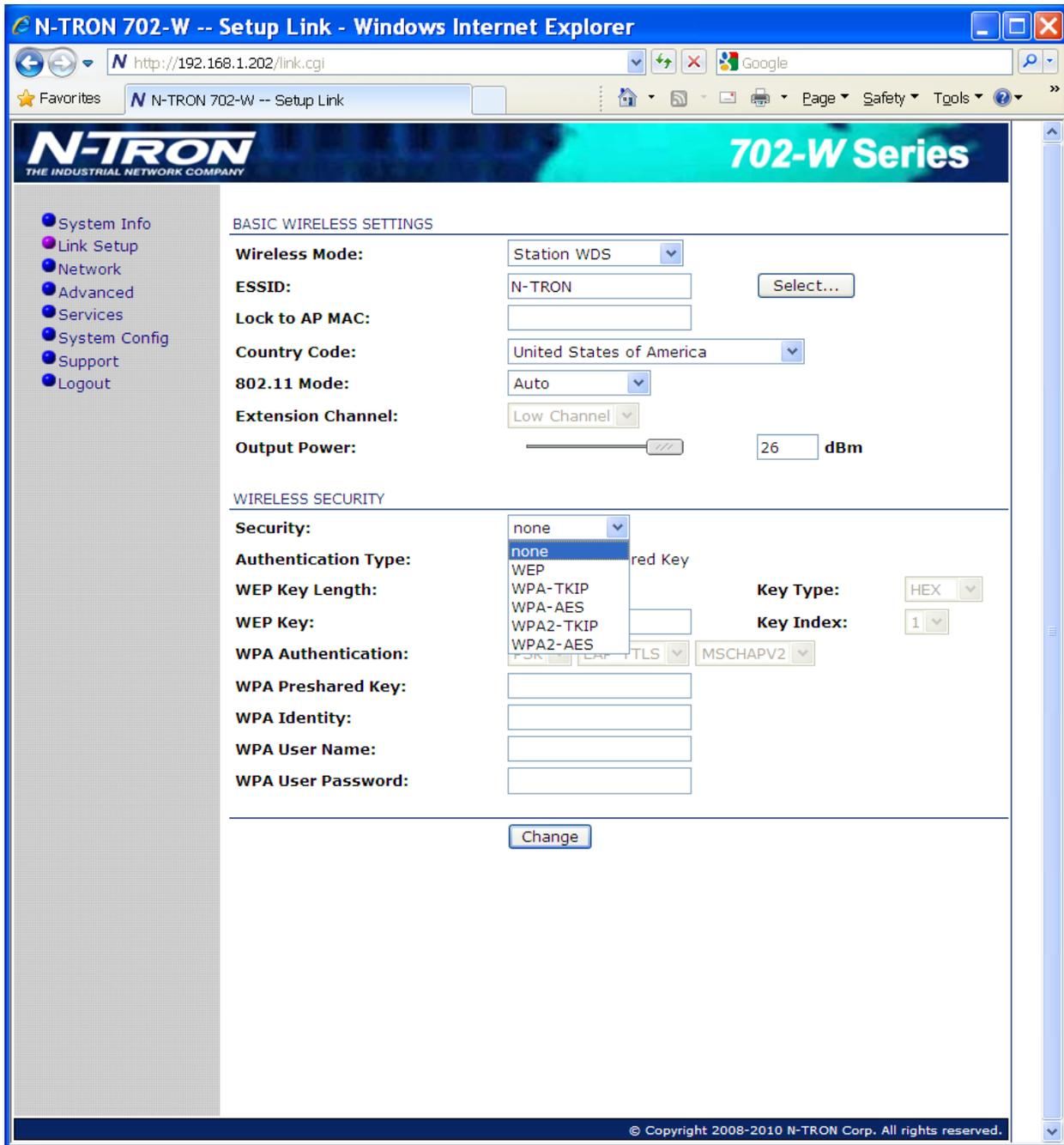
This section enables you to set parameters that control how the subscriber station associates to a wireless device and encrypts/decrypts data.
