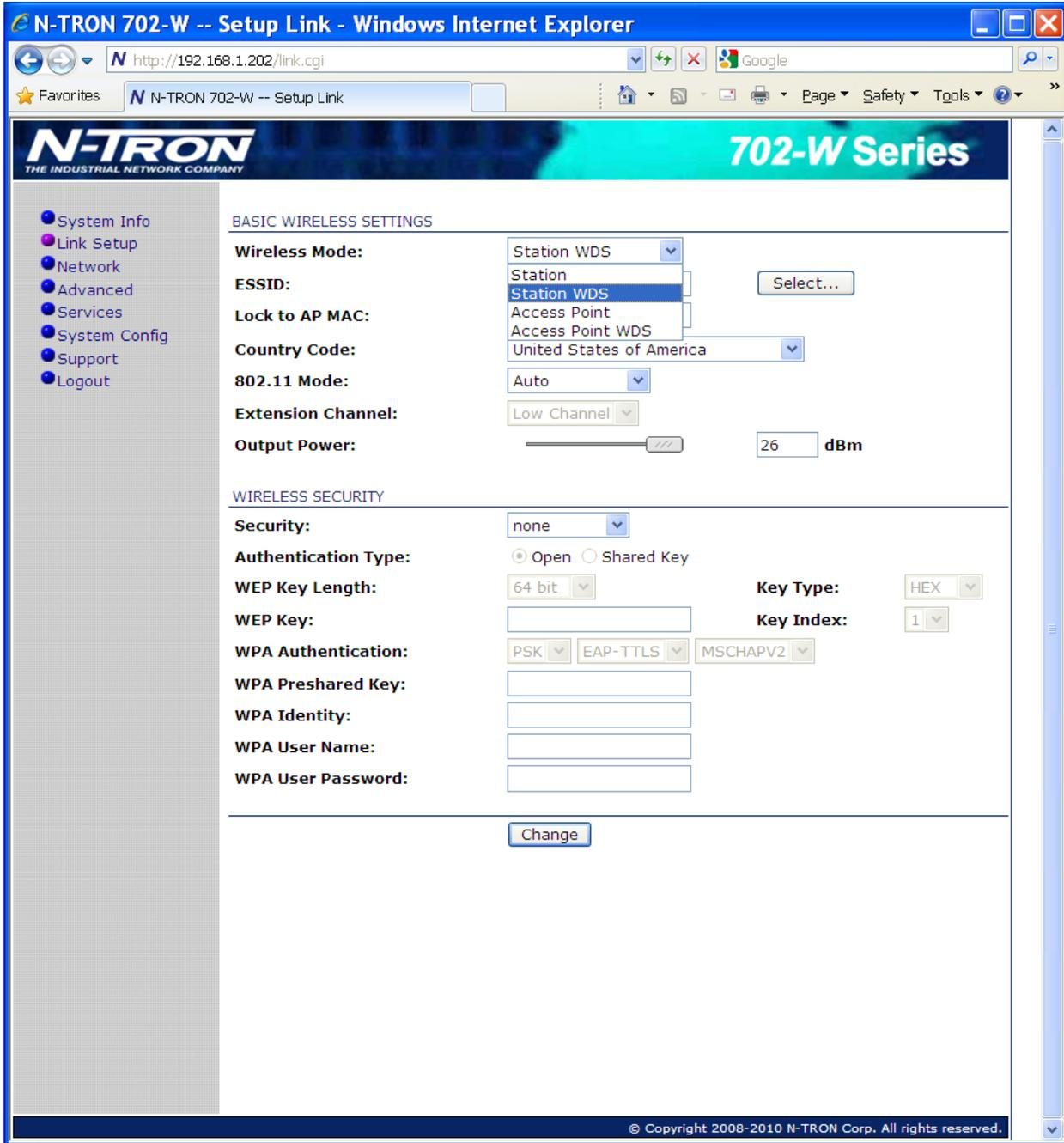
The Link Setup Page contains everything needed by the operator to setup the wireless part of the link. This includes regulatory requirements, channel and frequency settings, device mode, data rates, and wireless security.
