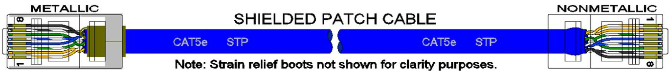
In the event all Cat5e patch cable distances are small (i.e. All Ethernet devices are located the same local cabinet and/or referenced to the same earth ground), it is permissible to use fully shielded cables terminated to chassis ground at both ends in systems void of low level analog signals.
