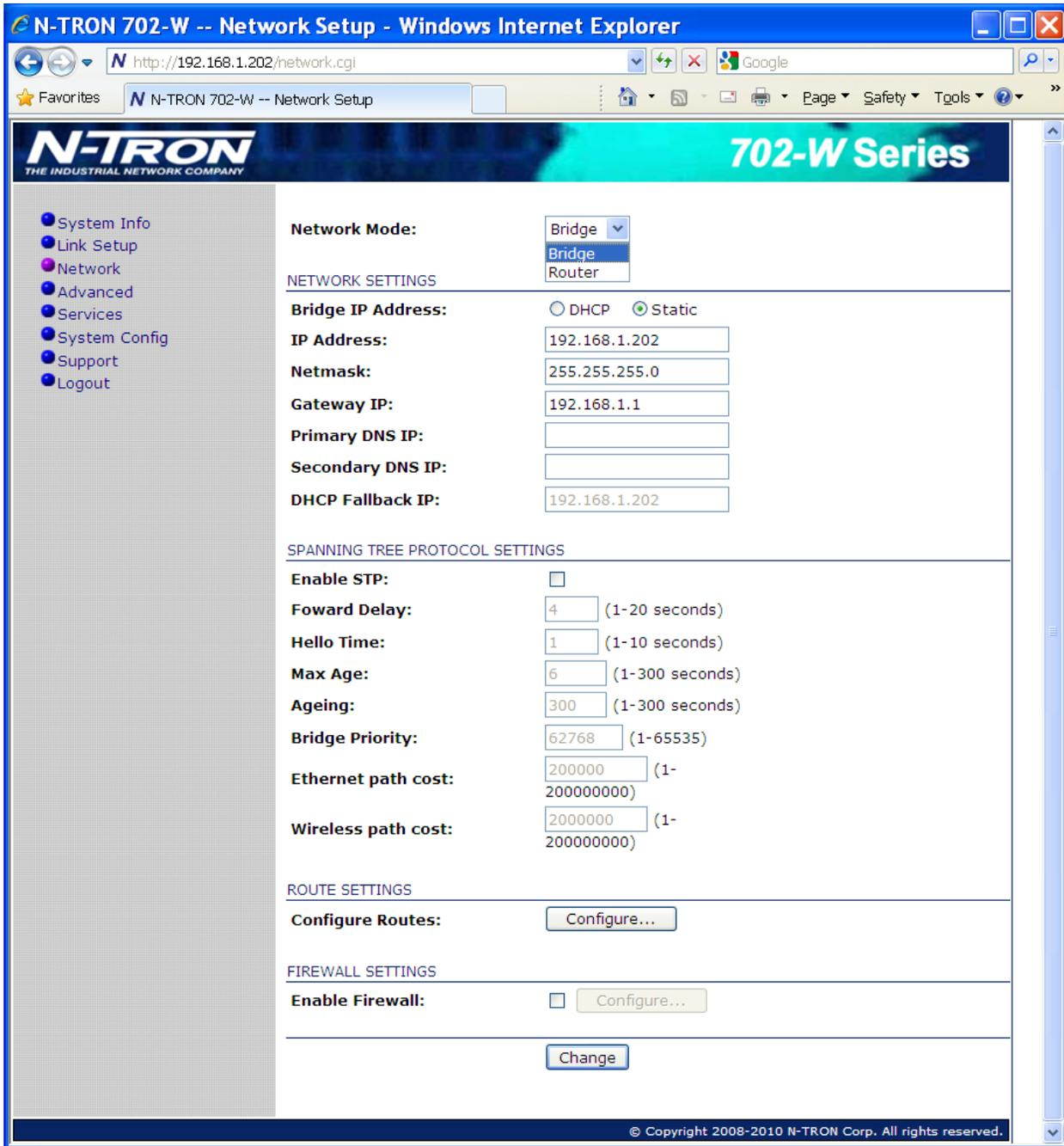
The Network Page allows the administrator to setup bridge or routing functionality.
