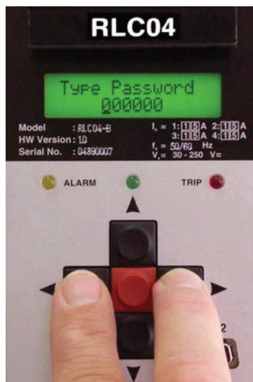
If a unique password has not been defined, no password will be requested and the display will switch straight to the Access PARAMETER SETUP menu screen in the main menu list.
