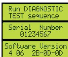
▼ Access the DIAGNOSTIC TEST sequence 2<sup>nd</sup> level screens.
