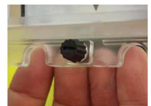
contacts of the fixed case. At this point, press the handle very firmly to fully insert the draw-out chassis. Then place the front cover by hooking the top catch over the clip on the fixed case. Align the front cover and refasten the bottom catch by a quarter turn.
