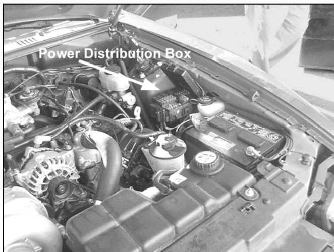
Fig. 1 - 2004 Ford Mustang Power Distribution Box location
