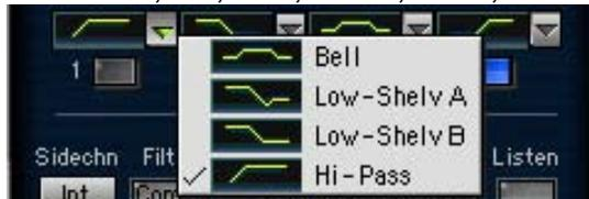
Determines the filter type for the related band. Clicking on the type display will toggle between the available types for each band. Clicking on the little arrow will display a pop-up menu with the available types to immediately select the type you need without toggling through the rest.
