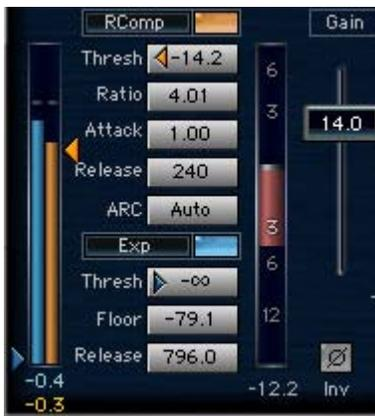
The Renaissance Channel Dynamics section consists of a Compressor, Gate and a "hidden" Clip Guard Limiter. Compressor related controls are Orange colored and the Gates' are Blue.
