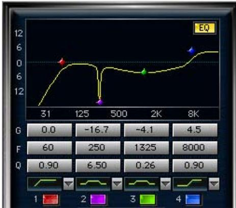
The Renaissance Channel EQ is a 4 band Paraphrastic Equalizer. Each band has 4 controls and an On/Off switch. The controls allow you to specify Type, Gain, Frequency, Q and each band. When a band is turned on its properties will filter the audio Input and its spectral Gain adjustment will register on the EQ Graph.
