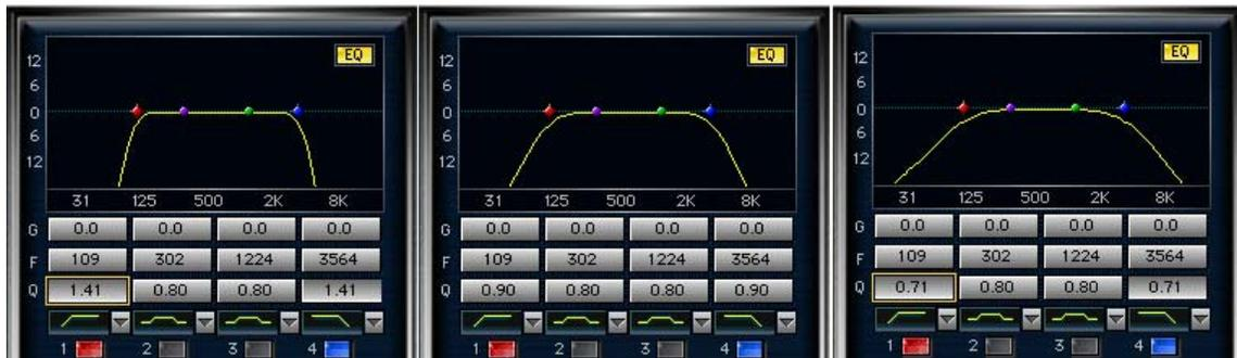
The cutoff frequency represents the point where the roll off is at -3dB. Only band 1 has the choice for Hi-Pass and only band 4 has the choice for Low-Pass.
