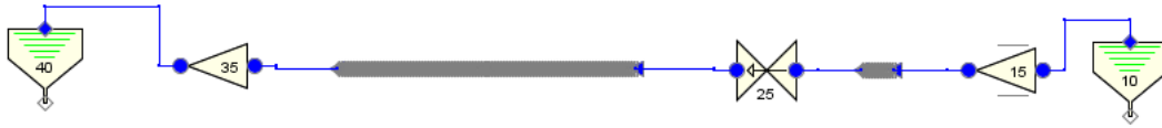
Figure 6.1: Model setup (in RELAP5) for studying the inertial swing check valve. A TIME-DEPENDENT JUNCTION (component number 15) is used in both codes for controlling the flow through the valve.
