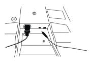
2. Connect the stereo audio cable from the Audio output of your sound card to the Audio Input of the monitor.
