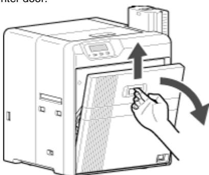
2 Press and hold down the cassette button, and pull out the retransfer film cassette (on the left) to remove the retransfer film.
