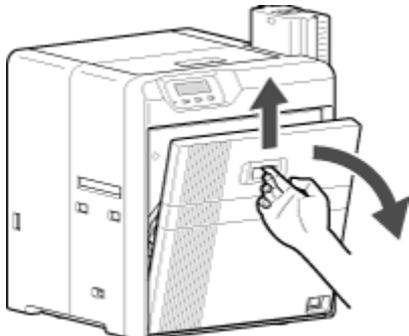
2 Press and hold down the cassette button, and remove the ink ribbon cassette (on the right) to remove the ink ribbon.
