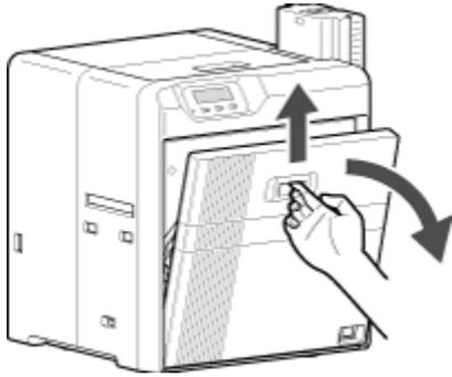
2 Press and hold down the cassette button, and pull out the ink ribbon cassette (on the right) to remove the ink ribbon.
