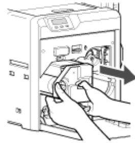
4 Apply alcohol to a cotton swab (large), and use it to wipe the four bobbin holders.
