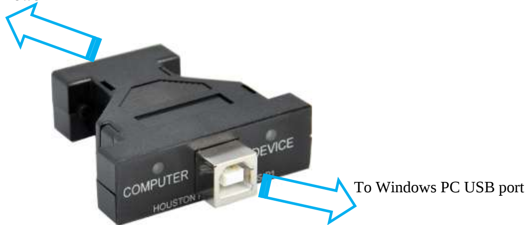
Houston Radar USB-RS-P1 USB powered RS232 interface to the radar.
