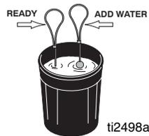
2. Agitate to mix, using a half-inch, variable speed drill with a mixing paddle, to a smooth, lump-free consistency.
