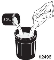
2. Agitate to mix, using a half-inch, variable speed drill with mixing paddle, to a smooth, lump-free consistency.
