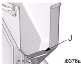
Before adding material to hopper, install burp guard (J). When only a small amount of material remains in the hopper, the burp guard prevents material from shooting out when the unit is turned off. This material could splash in the operator's eyes or on skin, or into the air.
