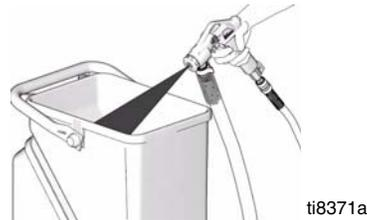
6. Spray water into a waste bucket to empty material hopper.
