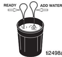
6. If the ball does not sink completely into the mixture within 10 seconds, add more water, agitate and try test again.
