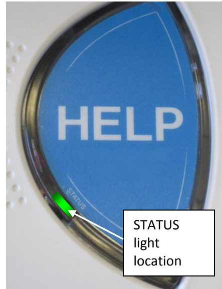
Figure 10. Status Light Detail
